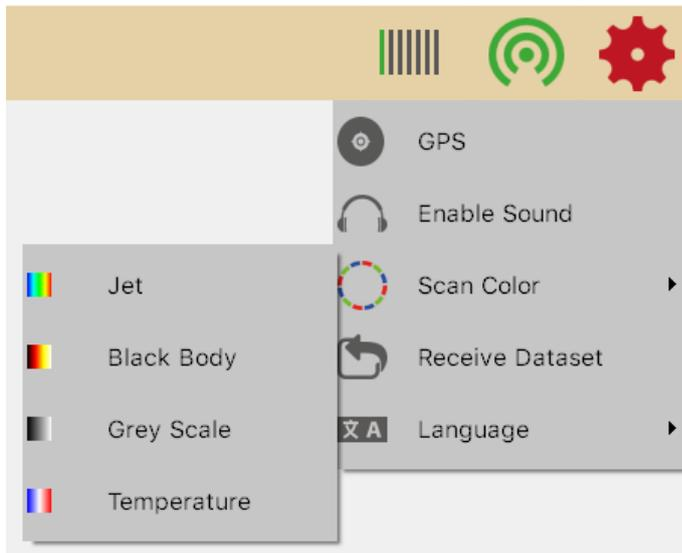
A colormap is a function, which turns the values of a dataset into colors. In TeroVido3D, the colormaps are represented by buttons depicting a color gradient. These color gradients correspond to the colormap. That means, the left color on the button corresponds to the smallest value which is shown.
